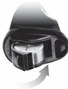
When your hearing instruments are not in use, open the battery compartment to prevent excessive battery drain and ventilate the instruments.
