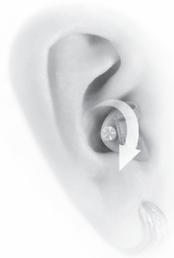
If your hearing instrument is equipped with a volume control wheel, place your finger on the wheel and rotate it forward (towards your nose) to increase the volume.
