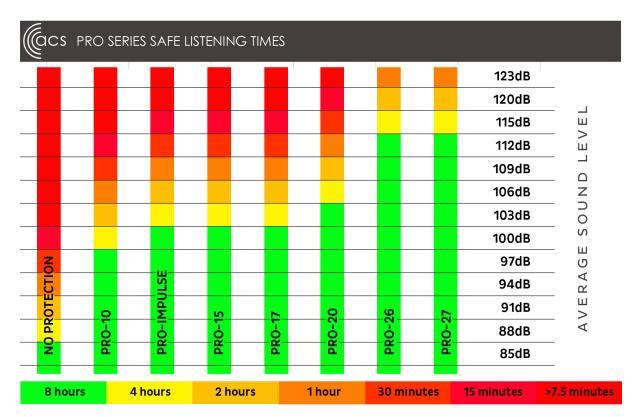
The above chart provides information showing approximately for how long and at what sound levels you can wear all the Pro-series hearing protection models safely. Pro-impulse also has protection against impulse sounds such as gunshot, explosions and sudden impact noise
